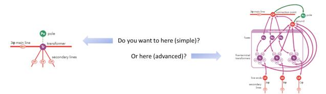
For example, you want to represent your transformer in a more detailed representation, rather than the single point that is in the current source data. Using the Assembly Builders, you can explode a single point and records in it's unit tables into a complex configuration.
